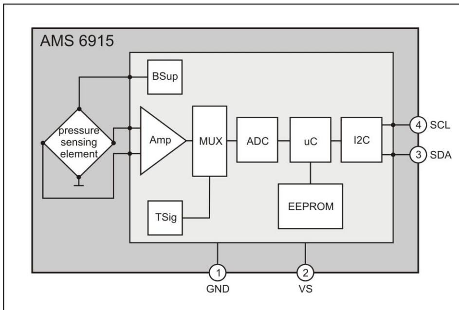
**Figure 1: Functional principle**
