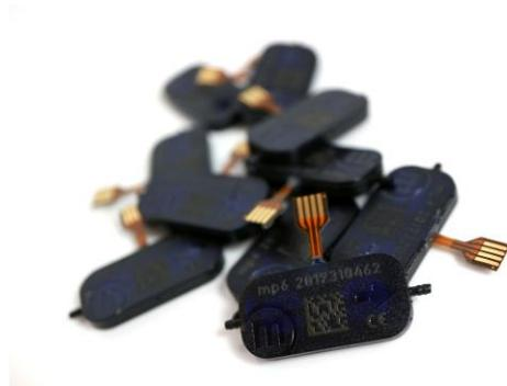
micropumps mp6-series used for various applications such as in medical technologies and analytics has been tested for different sterilization methods.
