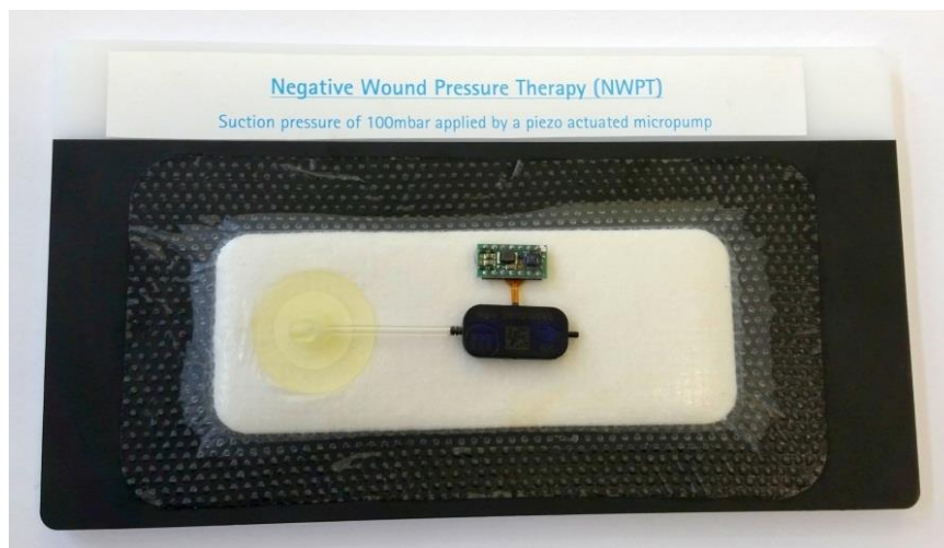
Figure 1: Wound pad with the mp6-AIR micropump and the mp6-OEM controller.
