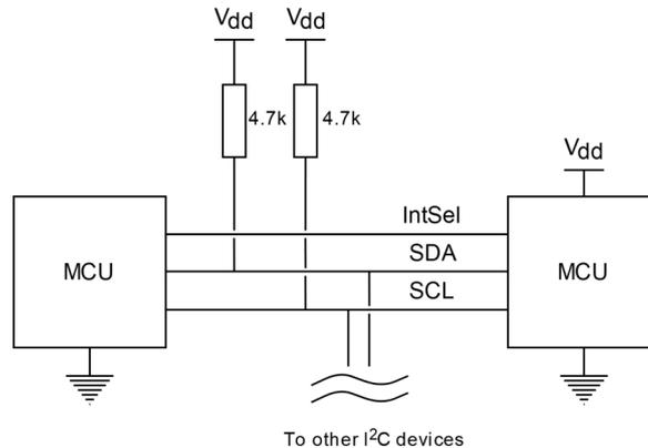
The sensors obey the full I<sup>2</sup>C protocol standard with the difference that they operate up to SCL (I<sup>2</sup>C Clock) speeds of 100 kHz. The sensors support clock stretching functionality. If the device is not ready to transmit data, holds the clock (SCL) line low and releases it once it is ready. The master must consider this condition and either identify it and wait until the clock is released or exit with a repeated start condition.
