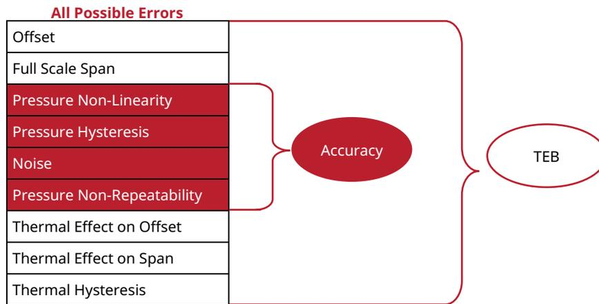
The figure below, illustrates the accuracy as well as the total error of the pressure measurement of ESCP-BMS1 sensors.
