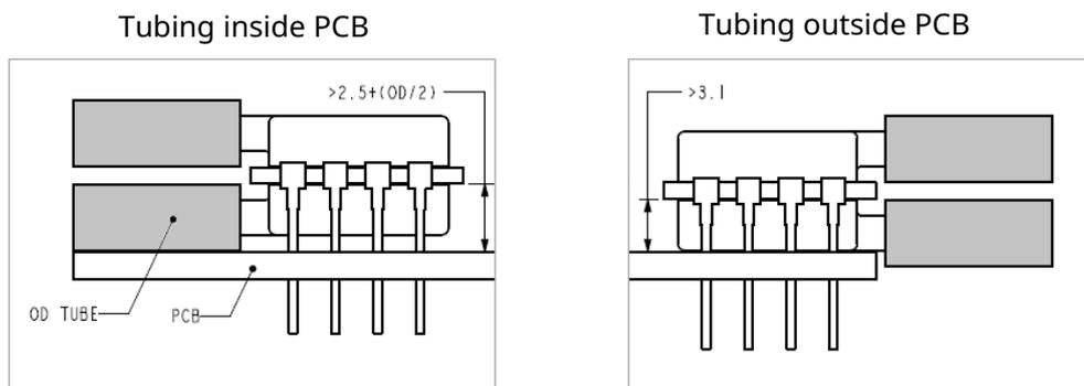
For optimal performance, ensure that the ESCP-BMS1 sensor is correctly mounted to the PCB as illustrated in the figures above. No mechanical stress should be applied to the sensor during or following its installation. The suggested internal diameter for the tubes is 2.5 mm.
