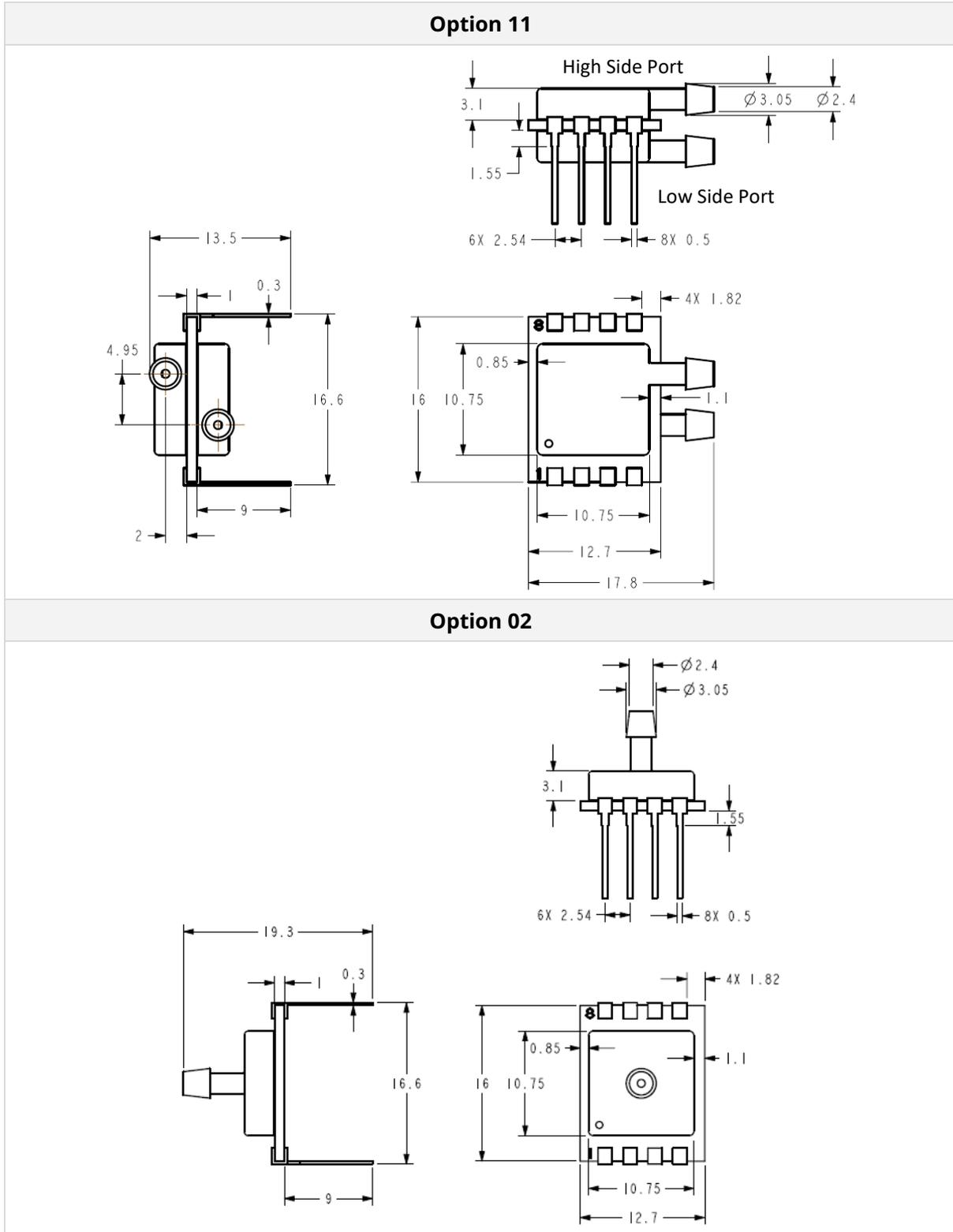
**16. Mechanical Drawings (mm)**
