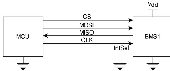
The sensor can communicate with two different serial interfaces, I<sup>2</sup>C and SPI (only one at the same time). The interface select pin selects which interface is active. Pulling the interface select pin high enables I<sup>2</sup>C interface whereas pulling it low enables SPI interface. In this document the SPI interface is described hence the interface select pin must be pulled low to operate in this mode.
