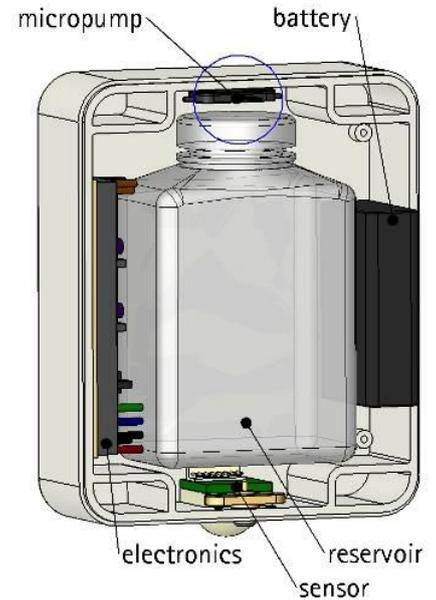
Despite its compact design, the dispenser housing includes a large reservoir and all functional parts.
