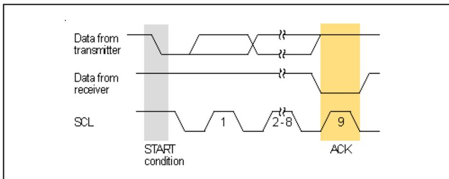
Fig. 7: Acknowledge (ACK) on the I<sup>2</sup>C bus
