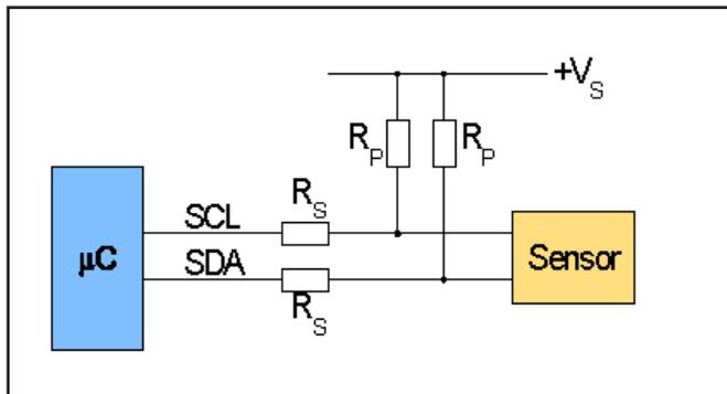
Fig. 12: I<sup>2</sup>C bus application circuit for HTD, HMI, HDI, HCLA, HCA and SSI pressure sensors
