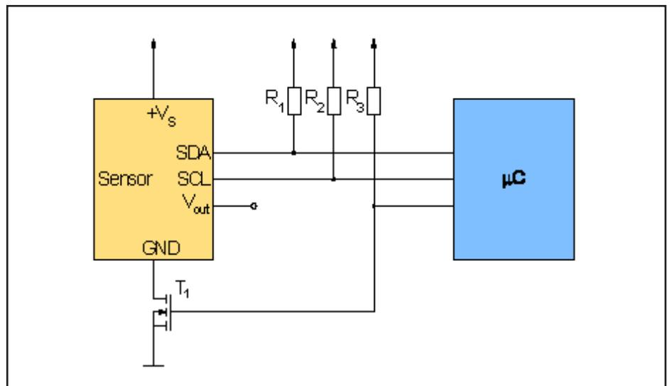
Fig. 13: Circuit for I<sup>2</sup>C reset
