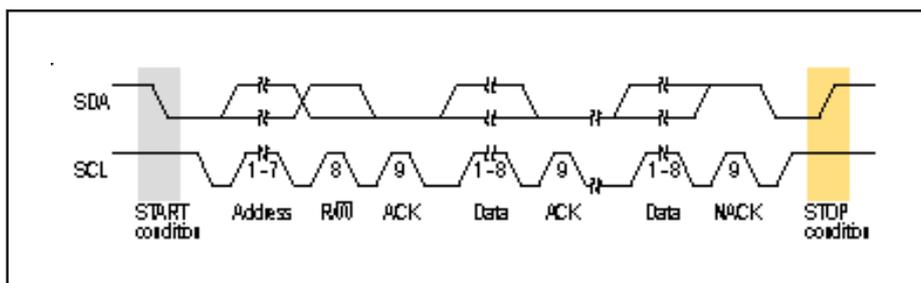
Fig. 8: Complete I<sup>2</sup>C bus data transfer
