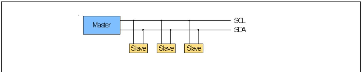
Fig. 1: Example of an I<sup>2</sup>C bus configuration
