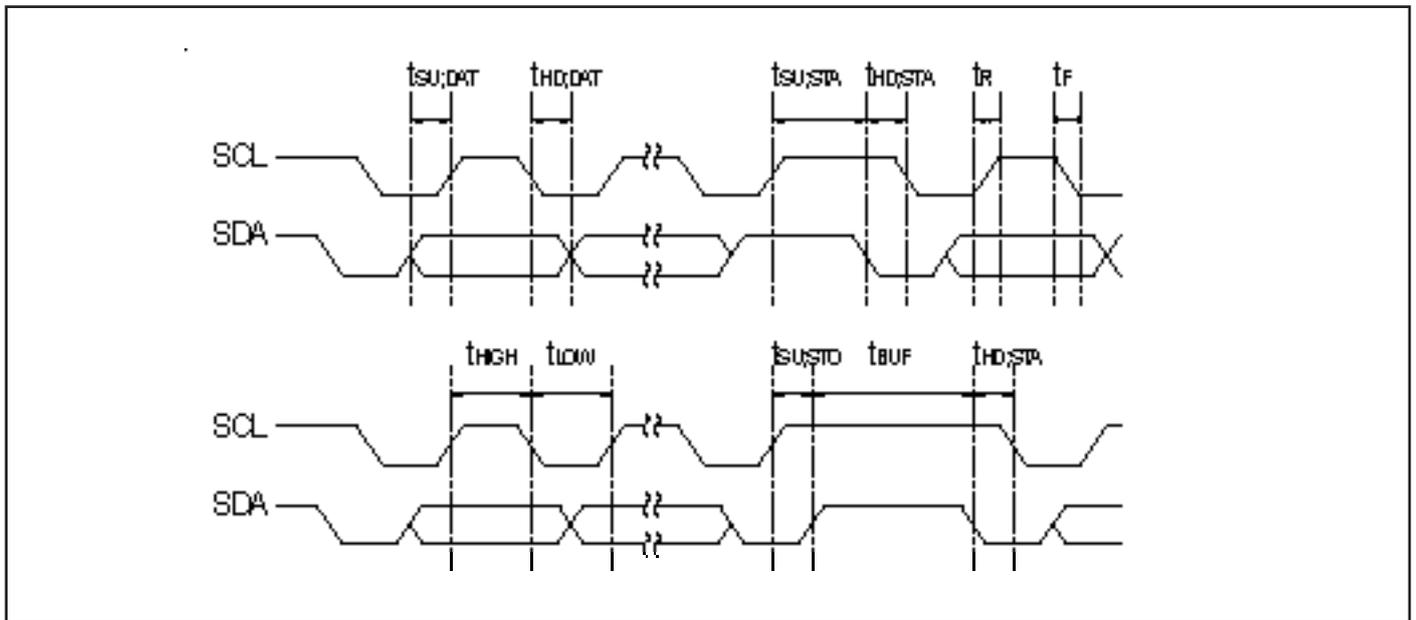
Fig. 11: I<sup>2</sup>C bus timing characteristics
