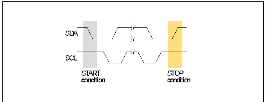
Fig. 4: I<sup>2</sup>C bus START and STOP conditions
